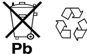
Labelling might vary due to application and dimension of the Battery. The manufacturer, respectively the importer of the batteries shall be responsible for placing at least the following symbols in accordance with International standards.
